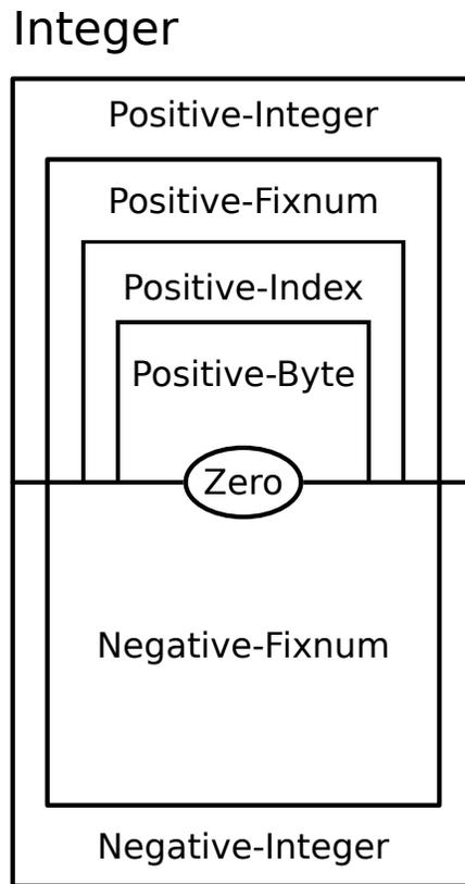
Like the previous diagram, types nested inside of another in the diagram are subtypes of its containing types.
