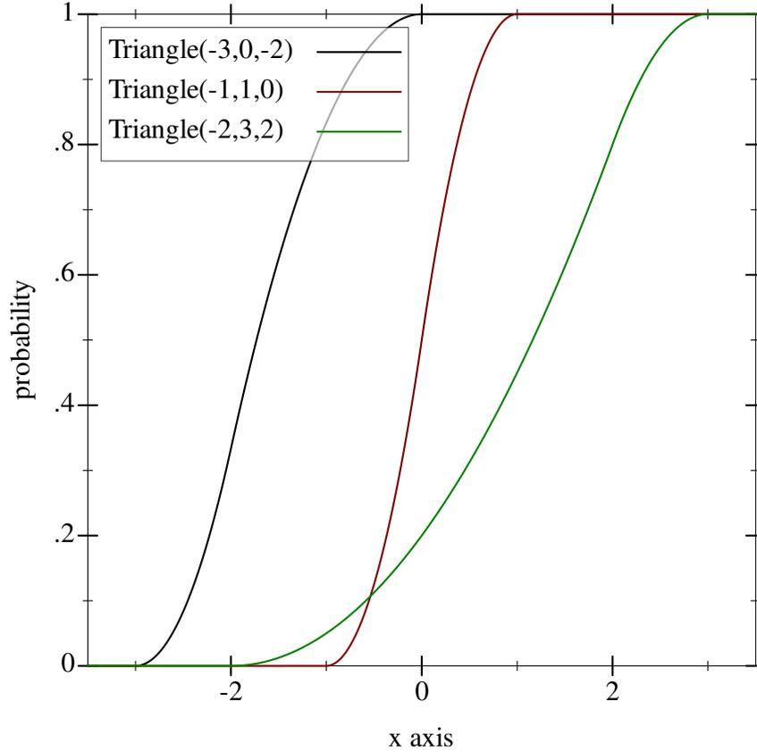
`(triangle-dist c c c)` for any real  $c$  behaves like a support-limited delta distribution centered at  $c$ .
