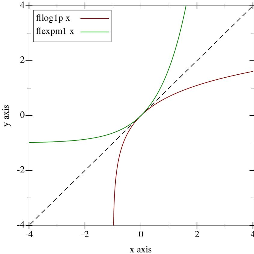
Notice that both graphs pass through the origin. Thus, inputs close to 0.0, around which flonums are particularly dense, result in outputs that are also close to 0.0. Further, both
