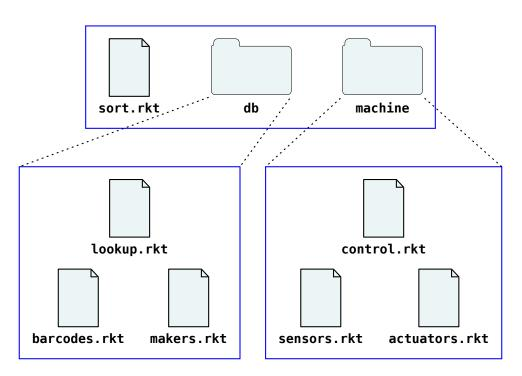
The "sort.rkt" module uses the relative paths "db/lookup.rkt" and "machine/control.rkt" to import from the database and machine-control libraries:
